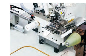
FR09 Fully Automatic Feeding, Position Adjustment, Pneumatic Extension Device
