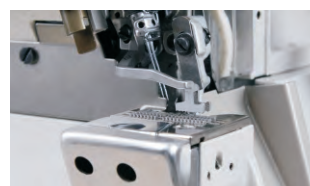
Differential feeding; Avoid of layers offset
