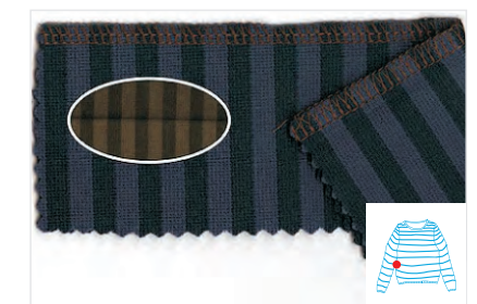
Four threads variable top feed
