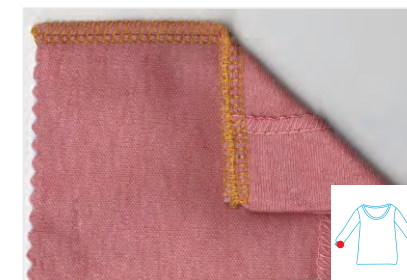
Four threads back latching stitch
