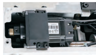
Cutter driven by servo motor
