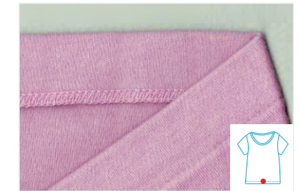
Three threads blindstitch hemming
