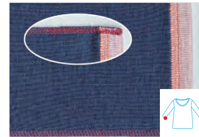
Three threads back latching stitch
