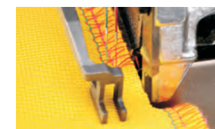
Differential feeding; Avoid of layers offset
