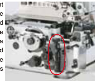
Differential-feed micro-adjustment mechanism
