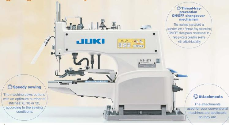
The single-thread, chainstitch, button sewing machine, which is frequently used for sewing buttons on men's wear and blouses under different sewing conditions, has been redesigned with its capabilities upgraded.
