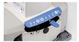
Stitch shape can easily be changed over between (3) and (3) button-hole configurations only by operating the lever. In addition, this single machine is able to sew two different kinds of buttons to save space and increase availability. (MB-1377)
