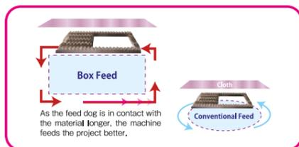
In order to provide beautiful seams and outstanding feed performance, Juki adopted box feed system. The conventional feed mechanism is oval motion. On the other hand, the box feed moves the feed dog in a box motion. This eliminates material shrinking and shifting. This accurate feeding system provides superior stitch quality for a variety of light to heavy weight fabrics.
