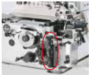
Differential-feed micro-adjustment mechanism
