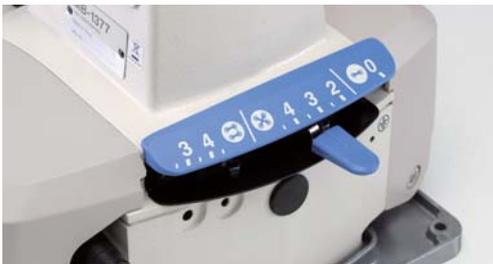
Stitch shape can easily be changed over between ⊗ and ⊗ button-hole configurations only by operating the lever. In addition, this single machine is able to sew two different kinds of buttons to save space and increase availability. (MB-1377)
